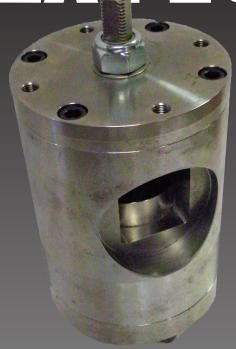
Flex Flow's revolutionary, cost-effective design makes it the **Next Generation Variable Port Valve.** Flex Flow's robust design ensures it will preform in the harshest of environments. The variable port allows for the flexibility to matchthe valve opening to the maximum flow range, yielding more precise control. The shaft and universal mounting pad are conductive to a variety of actuators, making it simple and easy to install.
