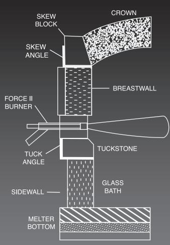
For most applications, mount the FORCE burner horizontally above the glass.
