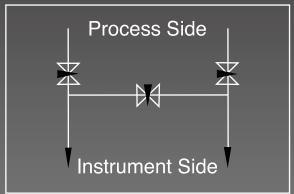
Ertl offers a series of 3 Valve Manifolds to isolate the different pressure instrument from the process by incorporating an equalizing valve with two isolation valves in differetal pressure applications.
